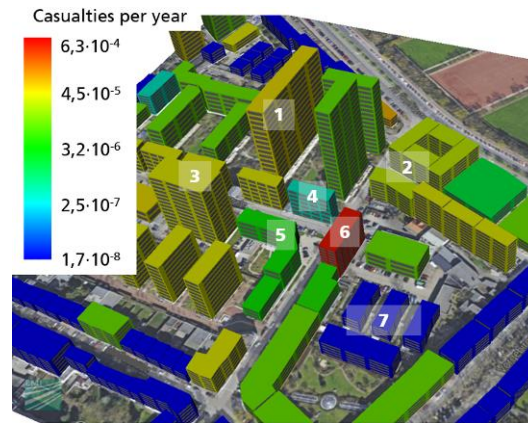
Figure 4. INACHUS approach 3D visualization of expected losses for weak spot identification with the VITRUV software for an explosive threat.
