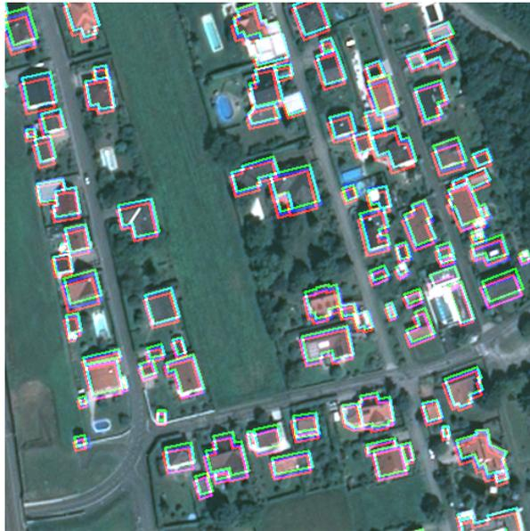
Figure 3: Green: groundtruth, red: misaligned, blue: aligned by the proposed method. When correctly aligned, the polygon has a cyan color.
